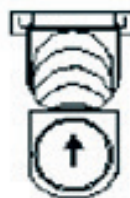
Open End Piece with 4" Pipe Connection Part.No.: CHG70011-20
